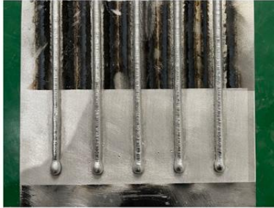
Cleaning of aluminum alloy after welding
