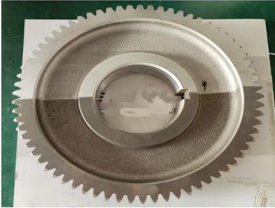
Gear surface rust
